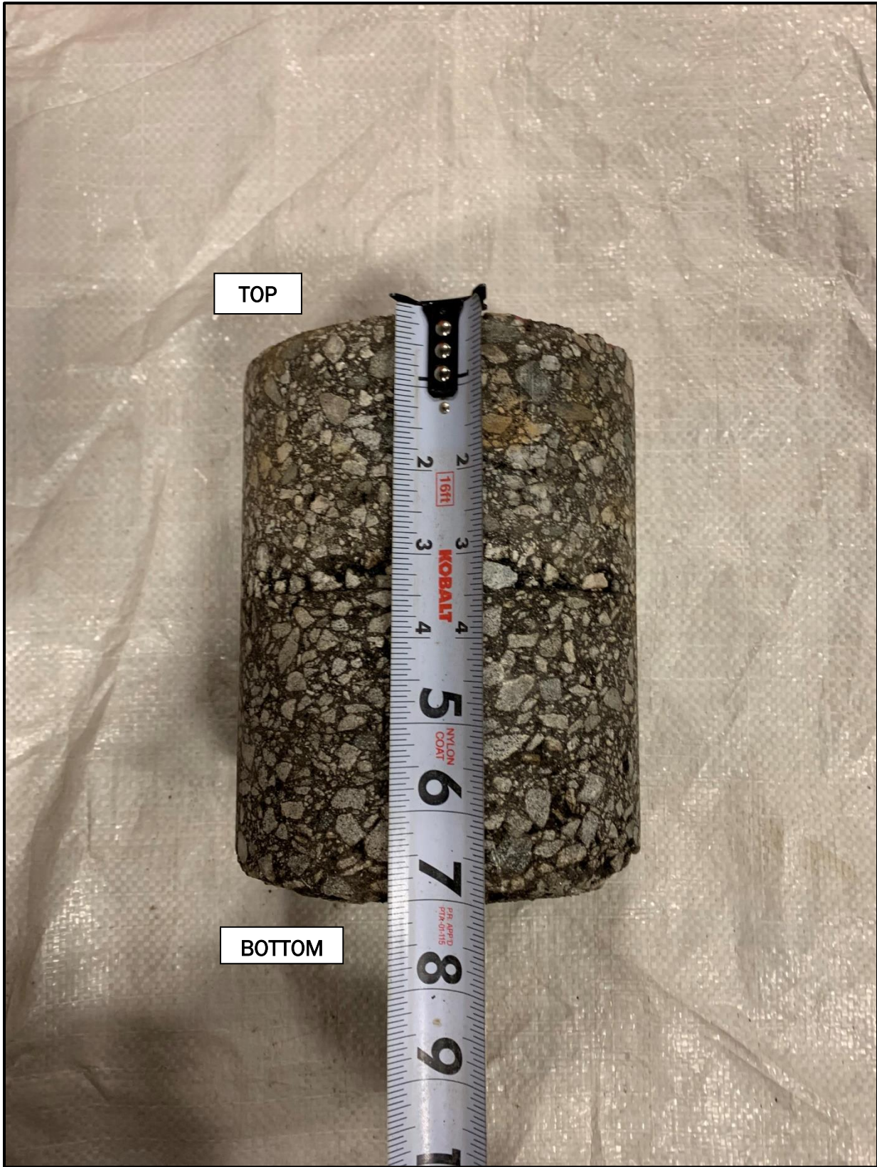
B-7 ASPHALT CORE PHOTOGRAPH 7" Asphalt 6 1/2" Graded Aggregate Base (approximate thicknesses)
